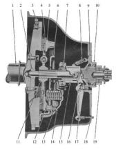
FIG. 21 -- CLUTCH ASSEMBLY
